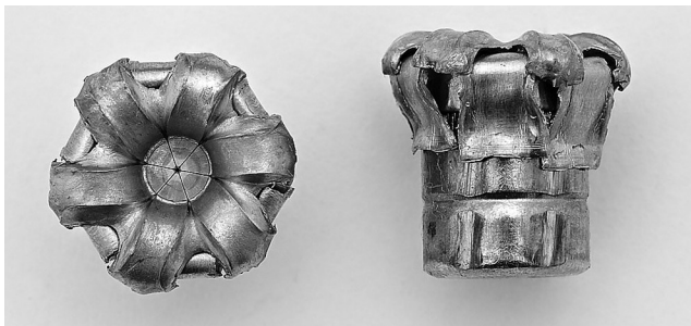
Figure 2.19 Hornady 9×19mm Critical Duty projectile that has passed through heavy clothing. The cartridge was a +P load. (Image courtesy of Hornady Manufacturing.)
